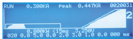
Run Screen – Constant power first pulse breaks through oxides.
