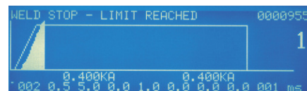
Run Screen – Shows termination of weld current during weld pulse.
