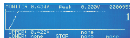
Monitor Screen – Shows weld current exceeding limit.
