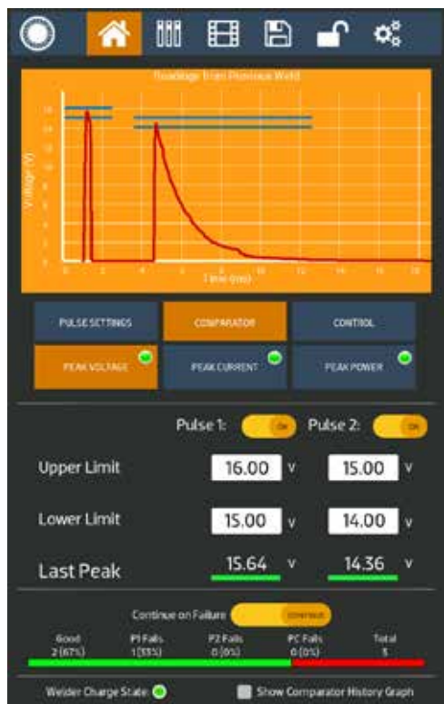
Figure 18.1. The Home Screen with the Comparator Tab and Peak Voltage sub-tab selected.
