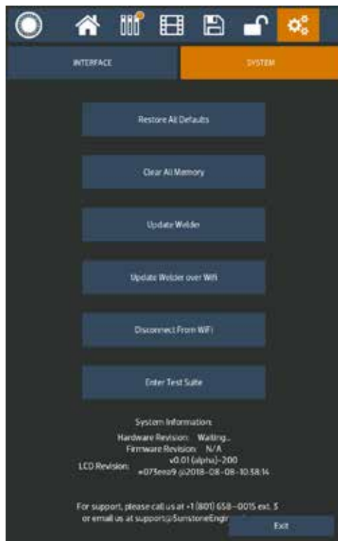
Figure 34.1. The Settings Screen can be used to make changes to the general power supply settings.
