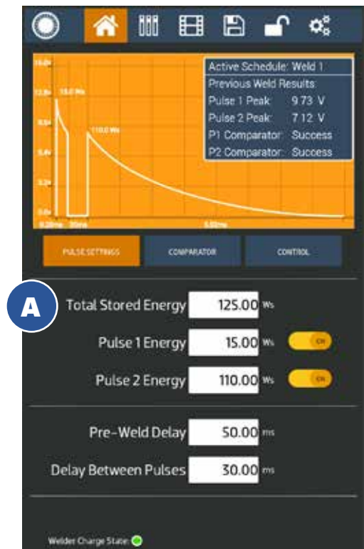
Figure 16.1. The Home Screen with the Pulse Settings Tab selected, which display energy values for the current weld.
