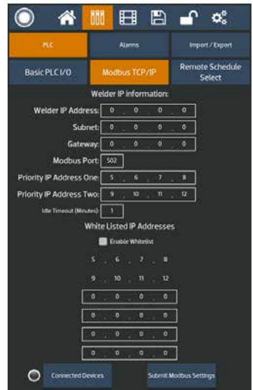
Figure 37.1. To configure an ethernet connection, access the Modbus TCP/IP screen by pressing the Communications Button, and then the PLC button.
