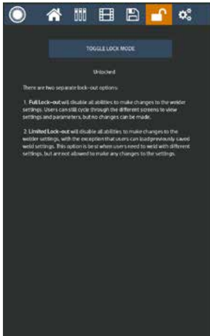
Figure 14.1. Use the Lock Screen to create/enter a password to lock the CDDP-A's weld settings. See Chapter 8 for more information.
