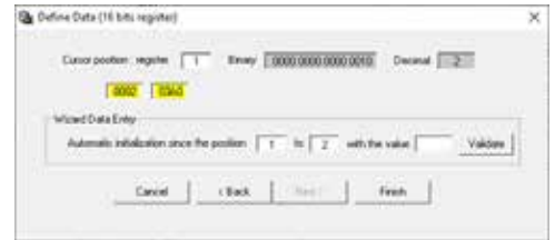
Figure 43.1. Use the Define Data window to convert a 32 bit register to 16 bit.
