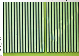
Less than 0.2 \mu\text{m} lines & spaces image (right) U-CFU combined with MX61 (below)
