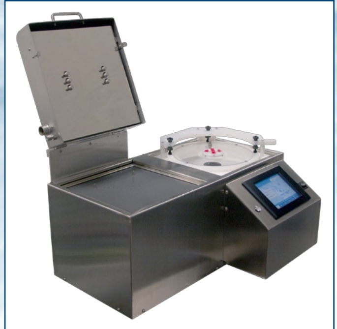
Cee® 200CBX shown with optional nitrogen diffusers on the bake plate
