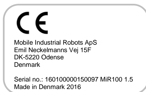
MiR100 identification nameplate example
