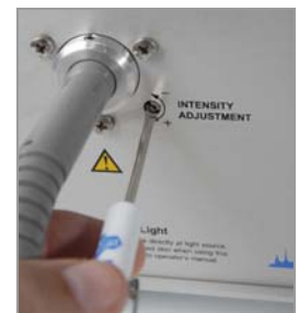
Intensity adjustment, with knob removed, performed with adjustment tool
