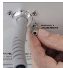
Intensity adjustment knob for fingertip adjustment
