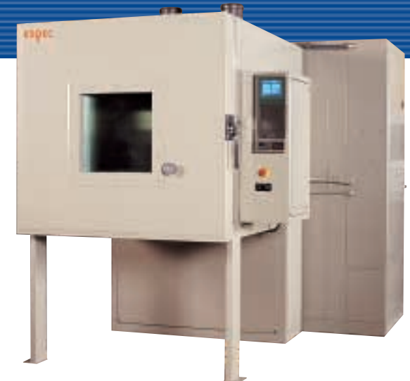
ET46-2CW (6.6'w x 10.6'd x 7.8'h exterior)
