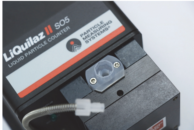
Figure 3-7 Tubing removed from capillary mount
