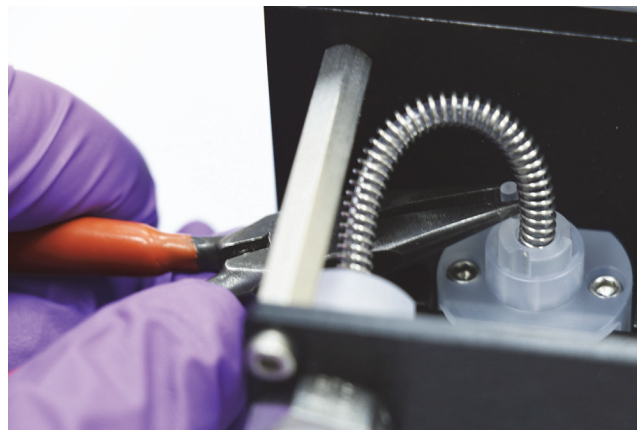
Figure 3-8 Locking pin removal from bottom capillary mount
