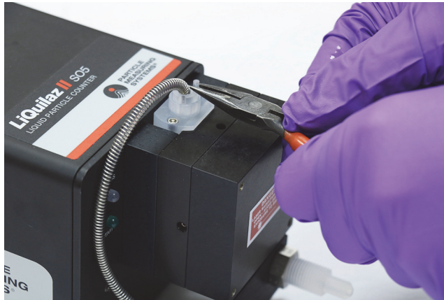
Figure 3-5 Locking pin removal
