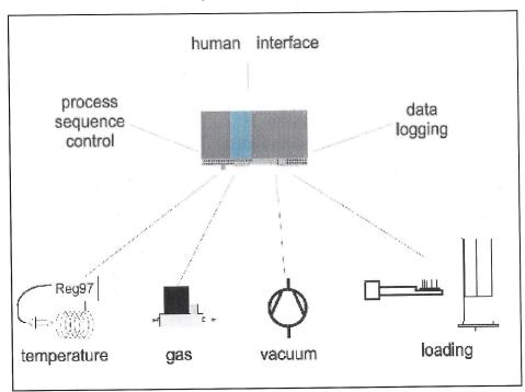
Each system is equipped with a control computer model CESAR including the CESAR-software. The control computer, an industrial PC, is independent of the Host-computer system. The control computer ie equipped with a field bus (CAN)-interface, HDD and a set of operation control systems (watchdog, over-temperature, etc.). The user interface for the tube computers and the handling computer of one furnace is a central color graphic, touch screen display.
