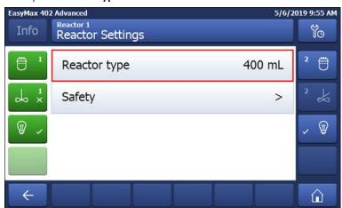
3 Select the reactor type that is installed.
