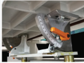
Tilting table with angle scale
