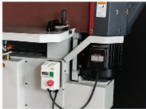
Powerful 3HP motor with oscillation gearbox
