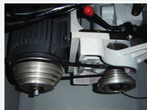
Powerful 7.5 HP motor with 5 spindle speeds
