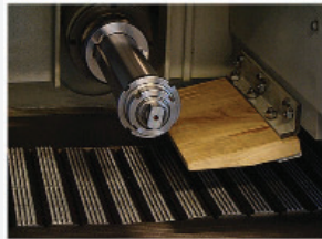
Precision cast iron chain, nickel chrome arbor with removeable saw sleeve
