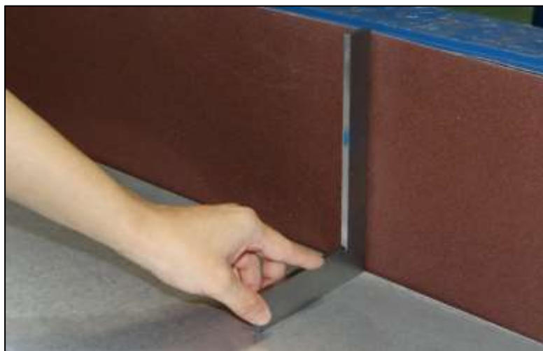
Figure 14. Setting main table to 90°
