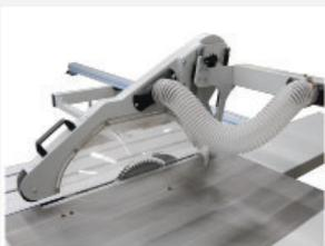
Overarm blade guard with quick change straight and bevel guards
