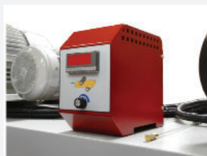
Inverter controlled variable planing speed
