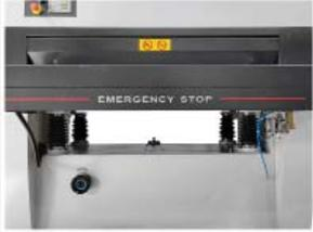
Four elevation screws
