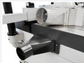
Dust ports located on the fence assembly and beneath the table
