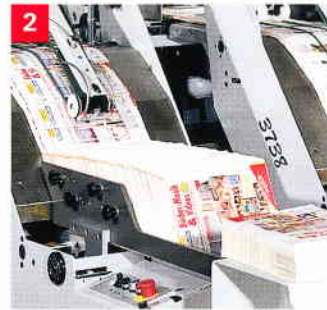
2 Streamfeeder loading without bundle extensions on flat pile feeder
