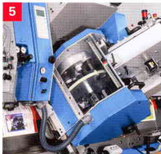
5 Sample gluer for tip-on product samples, cards, small brochures, CD-ROMs and Post-it® notes
