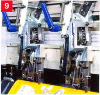
9 Stitching unit for standard, eyelet or child-safe stitching
