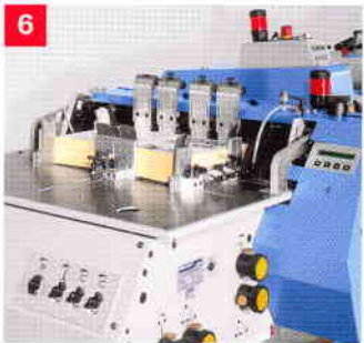
6 Cover/card folder feeder for folding single-sheet covers and cards
