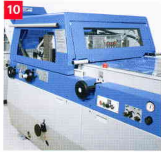
10 Three-knife trimmer for single, double and three-up productions as well as for various hole punching
