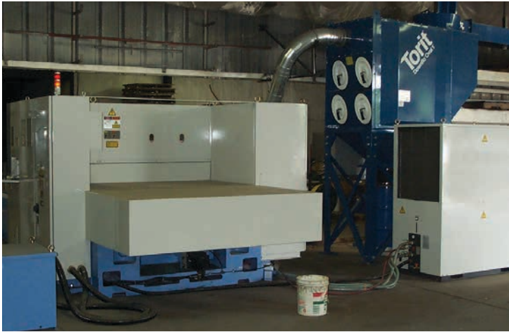
DFO on Laser Cutting 3,100 cfm (5,266 m 3 /h)
