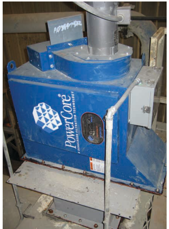
CPV - Feed Hopper 350 cfm (595 m³/h)
