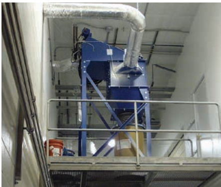
CPC on Milk Powder 1,200 cfm (2,038 m 3 /h)
