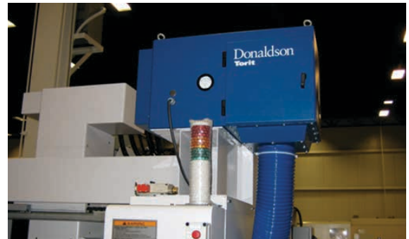
DMC on Wet Machining 390 cfm (662 m 3 /h)
