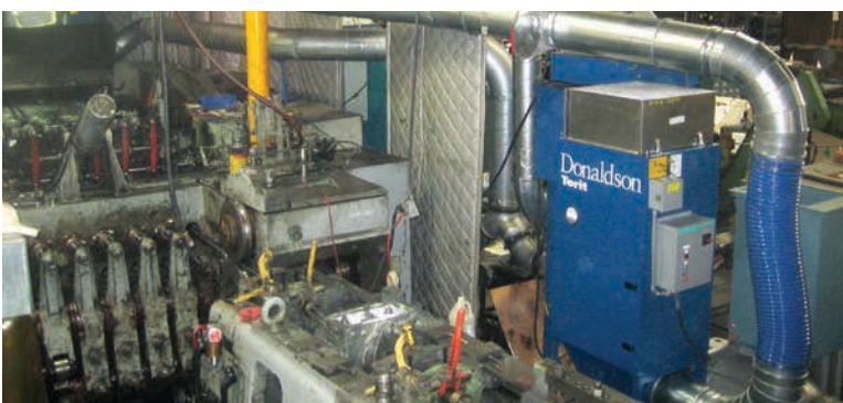
WSO on Cold Forming 1,200 cfm (2,038 m 3 /h)
