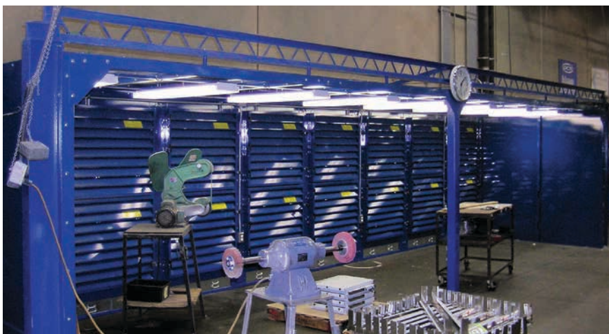
DWS on Custom Hand Grinding 38,500 cfm (65,398 m³/h)
