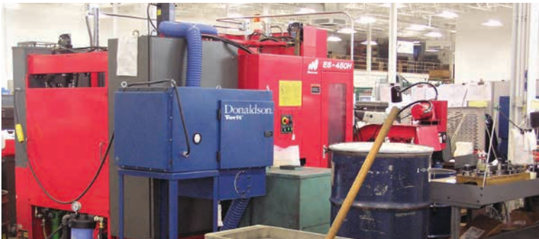
DMC on Machining 800 cfm (1,359 m 3 /h)
