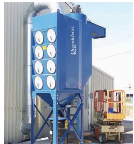
DFO on Plasma Cutting 5,000 cfm (8,493 m³/h)
