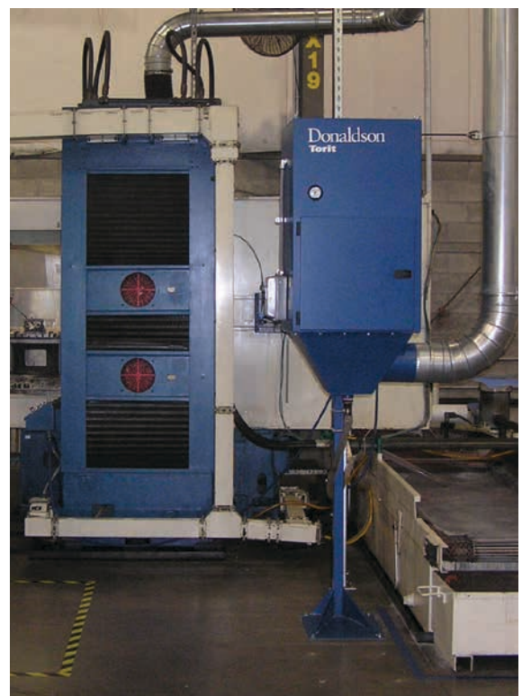
WSO - Horizontal Grinder 850 cfm (1,444 m 3 /h)
