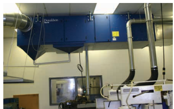
Modular Mediafilter™ on Grinding 2,000 cfm (3,397 m 3 /h)
