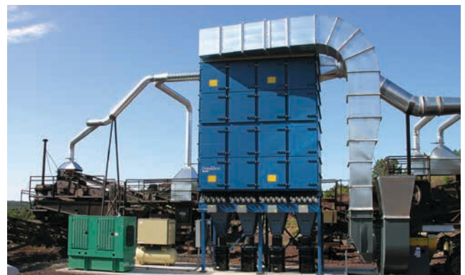
DLMC on Rock Crushing 41,000 cfm (69,645 m 3 /h)
