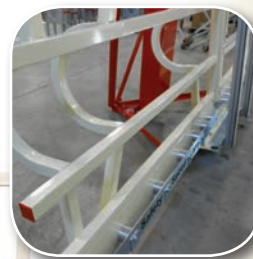
Frame Designed to Integrate Automated Stops
