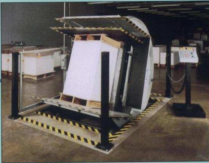
This Model A73VA is installed in a shallow pit for easy floor level loading using a standard pallet jack.
