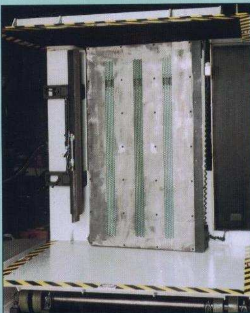
Air flow is directed through rows of holes in the air deck by narrow openings in the traveling air belt.
