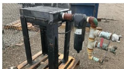
**Thermal Transfer Heat Exchanger**
