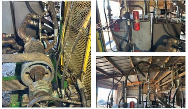
Part of entirety! Jack Shaft, Pumps Reservoirs, and Main Frame, Gear Flow Divider, 99 gallon capacity
