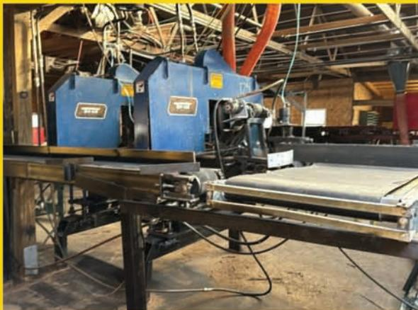
Coblentz Fabrication Double Head Resaw
