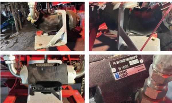
**Hydro-Leduc Hydraulic Piston Motor**
