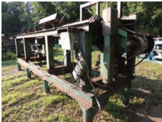
9997 LOG TROUGH $12,500.00 50"x 22' overall, air cylinder log clamp down, electric drive, WR124 chain w/cleats, air cylinder on loader 260-633-4047
