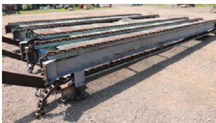
9043 $5,000.00 TRANSFER DECK 5 strand transfer deck, 12' 6" wide x 24' 6" long, electric drive, chains have rollers on top, good condition 260-633-4047
