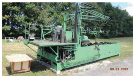
6031 $30,000.00 HMC DEBARKER rosser head style, all hyd. drive, 36" dia. log capacity x 12' long, very good condition 260-633-4047
