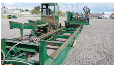
2087 $17,500.00 HMC 4 HEAD BLOCK CARRIAGE HMC HC-40, serial #330-1982, 4 head-block carriage, electric set-works, air powered dogs, 40' long track, was used with band head, includes cab, controls and log turner, complete unit ready to operate and in good condition 260-633-4047
