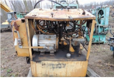
18210 $1,750.00 HYD UNIT used on Fulghum rosser-head debarker, 15 hp electric drive, 2 stage vane type pump, approx 45 gal tank, working condition 260-633-4047
