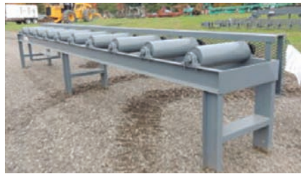
9129 $10,750.00 SUPREME MFG ROLLCASE 20" wide x 20' long, 6" dia rolls, 1 7/16" dia shafts, electric drive, BRAND NEW!! 260-633-4047
