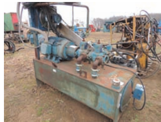
18186 $4,500.00 HYDRAULIC PACK 30 HP electric motor w/double pump direct mounter, approx. 100 gal tank, lots of electric control valves, oil cooler, electric control box 260-633-4047
