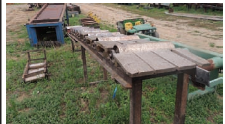
9070 $1,250.00 ROLL CASE 20" wide x 13' long, heavy duty 6" dia rollers, dead rollers, good condition 260-633-4047
