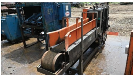
14067 $5,500.00 DEDUSTER Model: 450 LBD, SN: 23719L, 8" width capacity, electric drive, good condition 260-633-4047
