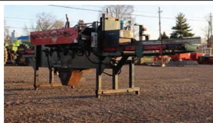
4035 $15,000.00 GANG SAW Morgan single arbor gang saw, capacity 12" wide x 5 1/2" thick, 75 hp electric drive on arbor, feed rolls are hyd drive, includes spare spacers, good condition and ready to work 260-633-4047
