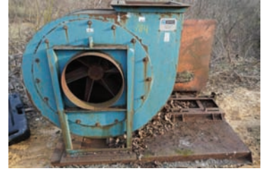
10346 $2,500.00 DUST BLOWER Koger dust blower, 38" dia, top discharge, 18" inlet/ 16" outlet, good condition 260-633-4047
