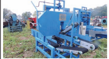
3079 $20,750.00 BAND RESAW single head resaw, 6" x12" cutting capacity, 28" dia band wheels, fast precision adjustment w/ mechanical counter, electric drive with VFD for feed belt, plug/play ready heavy duty construction, has return belt, BRAND NEW! 260-633-4047
