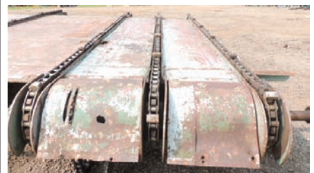
9042 $3,500.00 TRANSFER DECK 4 strand transfer deck, was used as incline deck, 12' wide x 12' 6" long, electric drive, 81X type chain with lugs, good condition 260-633-4047
