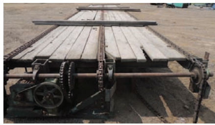
9057 $12,500.00 GREEN CHAIN 3 strand green chain, 8' wide x 101' log, electric drive, 81X type chain, good condition 260-633-4047
