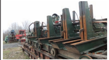
2078 $42,500.00 CLEEREMAN 4 HB MILL Cleereman 4 head block , Model 40, air over air setworks, includes cab/track-frame/ carriage drive and all controls, in good working condition 260-633-4047
