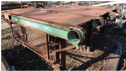
9664 $3,000.00 TRANSFER DECK 4 strand, 10' wide x 11 1/2' long, electric drive, H-78 chain, good condition 260-633-4047
