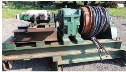
18197 CARRIAGE FEED & DRIVE $7,500.00 Tyrone Berry SN: A2850, Model:SMA-225, spool of 3/4" steel cable, 60hp electric motor, hyd tank, good working condition 260-633-4047
