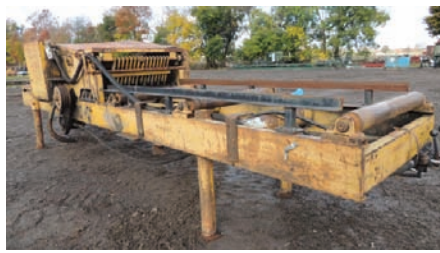
5119 $7,500.00 EDGER Edmiston 4" thick x 28" wide capacity, 2 movable blades, includes infeed/outfeed, hyd movable blades, good working condition 260-633-4047
