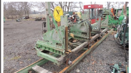
2086 $12,500.00 CIRCLE SAWMILL Frick 4 head-block carriage, only 2 head-blocks have dogs, electric set-works, includes husk, track/ frame, drive and all controls, good working condition 260-633-4047
