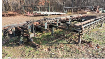
3081 $8,500.00 RESAW RUN-AROUND Morgan complete run-around system for single head resaw, 8' wide x 25' long over-all, 14" wide rollers, hyd drive, hoses will need to be replaced, working condition 260-633-4047
