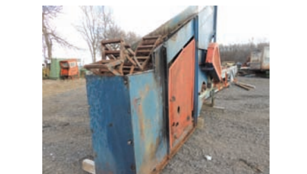
9852 $3,500.00 WASTE CONVEYOR ladderback chain, 18" wide pan x 33' long, 12" sides, electric gear box drive, was used on incline, good condition 260-633-4047
