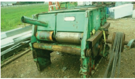
5089 $15,000.00 SHURMAN GANG EDGER 6"x42" wide overall, includes infeed and outfeed rollers, working condition 260-633-4047
