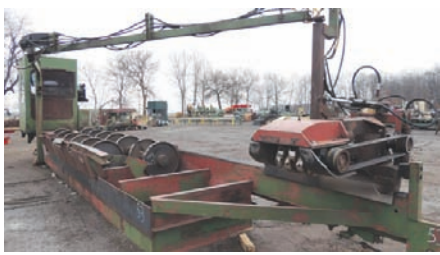
6044 $32,500.00 DEBARKER Mellott roller-head debarker, electric drive, hyd cylinder for head up-down, recently in production and in good operating condition 260-633-4047
