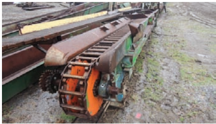
9063 $12,500.00 LOG TROUGH 30' long, 12" wide ladderback chain, electric gear box drive, 1 set of log kickers, good condition 260-633-4047
