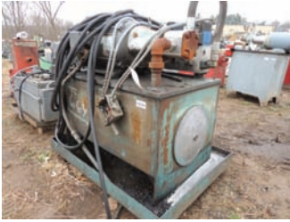
18224 $1,750.00 HYD POWER UNIT 15 hp electric power, vane type pump, includes 4 electric valves, approx 60 gal capacity, very good condition 260-633-4047
