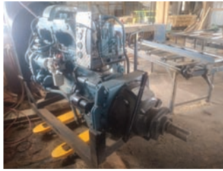
12136A $8500. OBO 855 BLOCK CUMMINS DIESEL POWER UNIT 290 hp, turbo, 2 7/16" stub shaft. Single 14 clutch, IN GOOD condition, was used on the mill 660 280 5110
