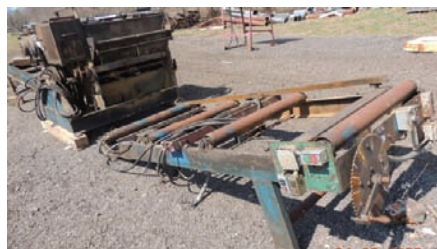
5111 $15,000.00 CORNELL EDGER 6" x 42" capacity, MN: HE42, SN: 703-10-81, single arbor, (4) 19" saws, 2 movable blades, 8" infeed, 8' powered outfeed, electric drive, comes w/ spare spacers, saws and laser lights 260-633-4047
