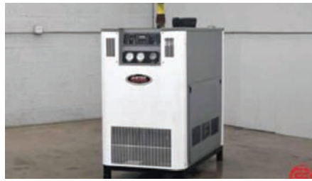
18193 AIRTECK CT400 AIR DRYER $1,750.00 Air-Tek refrigerated air dryer, 400 CFM, 2hp, 460 volts, excellent condition 260-633-4047
