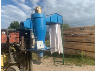
10342 $1,500.00 CYCLONE dust cyclone 20" dia x 5' tall, 6" inlet, electric drive, includes bag house, good working condition 260-633-4047
