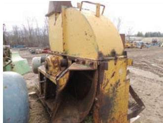
7138 $15,000.00 CHIPPER Fulghum 6 knife chipper, 60" dia, top discharge, working condition 260-633-4047
