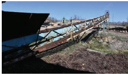
9025 $8,500.00 PADDLE CHAIN CONVEYOR 3" x 13" paddles, 16" pan, 15" sides, electric drive, 20" x 68' long, good condition 260-633-4047
