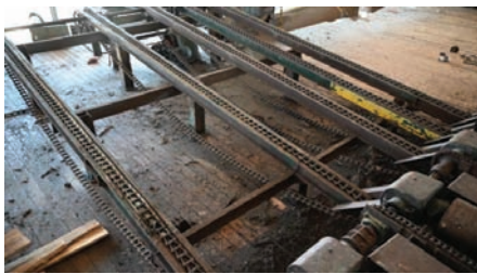
9018 $4,000.00 TRANSFER DECK 5 strand, 13' wide x 18' 6" long, H78 chain, electric drive, air cylinders on pop up board stop, good condition 260-633-4047
