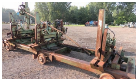
2083 CLEEREMAN 363+CARRIAGE SN: 36-307, MN: 36, 3 head block, air dogs, tapers, setworks, 16' long, 50" wide center to center wheels 260-633-4047
