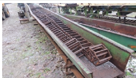
9132 $6,500.00 WASTE CONVEYOR 24" wide pan x 73' long, electric drive, ladder-back chain, working condition 260-633-4047
