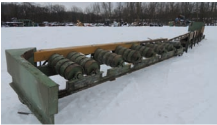
9127 $6,500.00 ROLL CASE 24" wide x 32' long, 10" dia rollers, spiral rolls on one end, electric drive, heavy duty and in very good condition 260-633-4047
