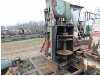
5097 $7,500.00 VERTICAL EDGER 3 blades, 2 movable, 50hp electric drive, 6" capacity, good condition 260-633-4047
