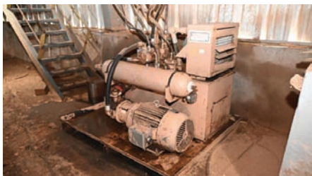
18199 HYD UNIT $3,750.00 40 hp electric, approx 150 gal capacity tank, PVR50 hyd pump, includes all valves attached, very good condition 260-633-4047
