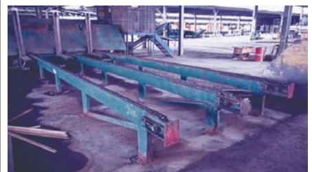
9054 $6,000.00 TRANSFER DECK 3 strand transfer deck, 11' wide x 27' 6" long, electric drive, 81X chain, good condition 260-633-4047
