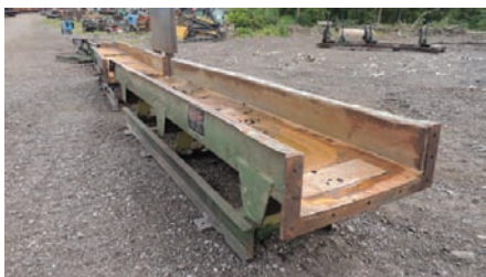
9066 $15,000.00 VIBRATING CONVEYOR Mellott 24" wide pan x 50' long, 8" sides, includes sawdust section and chipper mouth, hyd drive, good working condition 260-633-4047
