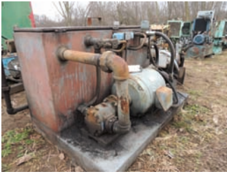
18110 $2,500.00 HYDRAULIC UNIT 15 HP. electric drive, 2 pumps, several electric valves, good working condition 260-633-4047
