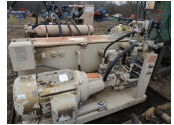
18153 $3,500.00 HYD. UNIT GS hyd. unit, 25 HP. electric drive, 2 pump sections, one is a pressure compensated, very good condition 260-633-4047
