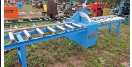
17094 $8,625.00 CHOP SAW Pro-Cut chop saw, up-cut style, 7" x9" cutting capacity, 22" dia blade, includes 8' infeed/outfeed, 4 flip stops, BRAND NEW, buy this one or order one to your specs 260-633-4047
