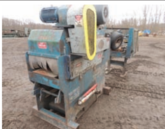
14056 $10,000.00 SIZER Brewco Model; BR-413, 14" wide x 6" tall capacity, 40hp electric drive, good condition 260-633-4047
