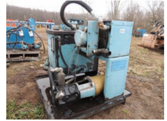
18213 $1,750.00 HYD UNIT 5 hp electric drive, pressure comp pump, cooling radiator, approx 30 gal capacity tank, good condition 260-633-4047
