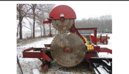
2090 $7,500.00 CIRCLE SAW HUSK Circle saw husk, used with a Corinth mill, 56" bottom blade-36" dia top blade, 150 hp 1180 rpm's electric drive, air clutch for top saw, off-bearing belt, excellent condition 260-633-4047
