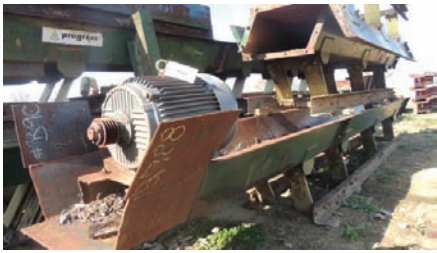
9985 VIBRATING CONVEYOR $30,000.00 93' long, electric drive, 9" tapered sides, 18" pan at bottom, 26" at top, includes chipper infeed and fiberglass sections, good working condition 260-633-4047
