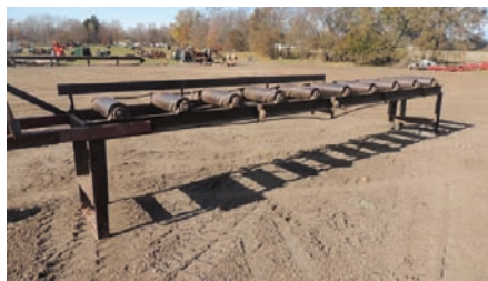
9088 $3,000.00 ROLL CASE 24" wide x 20' long, 7" dia rolls, no drive, good condition 260-633-4047
