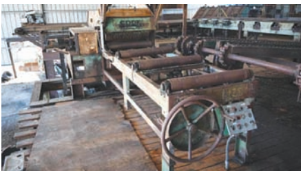
5114 $9,500.00 COOK EDGER Model:36EZTD, SN: 42, 5" x 21' tailing belt outfeed, 38" x 9' infeed rolls, 6" x 36" infeed cap, control panel, manual blade set, (2) 20" blades both are adjustable, electric drive, good heavy duty older unit 260-633-4047
