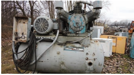
18227 $3,200.00 AIR COMPRESSOR piston type compressor, 3 stage, 25 hp electric motor, approx 80 gal horizontal tank, working condition 260-633-4047
