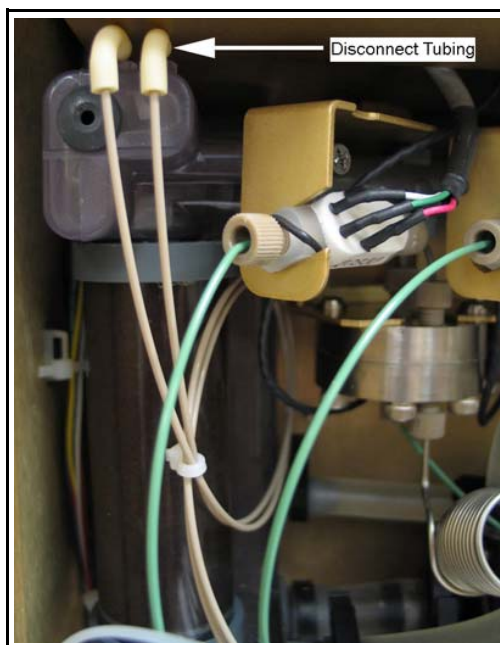
Figure 40: Disconnect the Tan Tubing that Connects to the DI Water Reservoir
