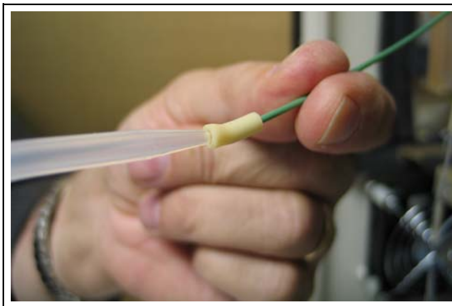
Figure 44: Draining the Measurement Module
