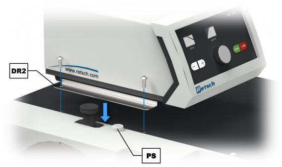
Fig. 36: Mounting the vibratory feeder DR 100
