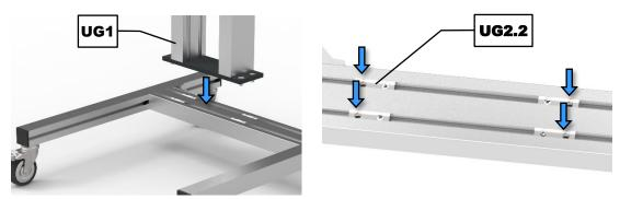
Fig. 10: Positioning the base
