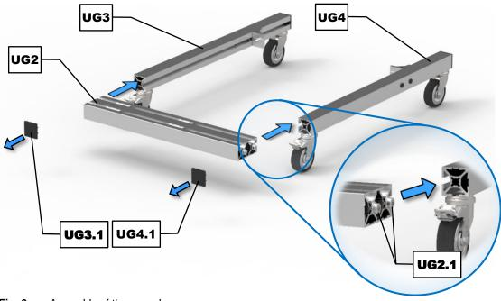
Fig. 6: Assembly of the cross bar
