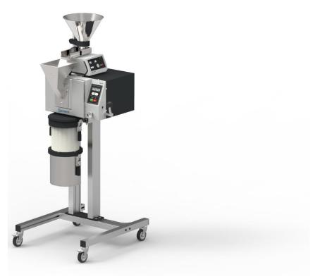
Fig. 34: SR 300 with vibratory feeder DR 100
