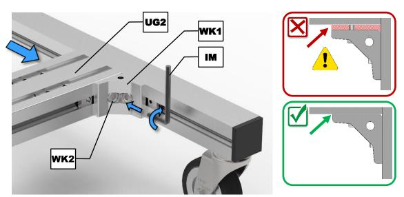
Fig. 7: Attaching the cross bar to the brackets
