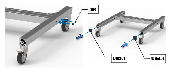
Fig. 9: Installing the protective caps and covers
