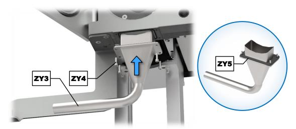
Fig. 41: Installing the cyclone adapter
