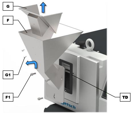
Fig. 31: Cleaning the feed hopper
