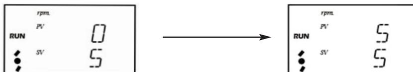
(3) Run time can be verified during shaking if you press
