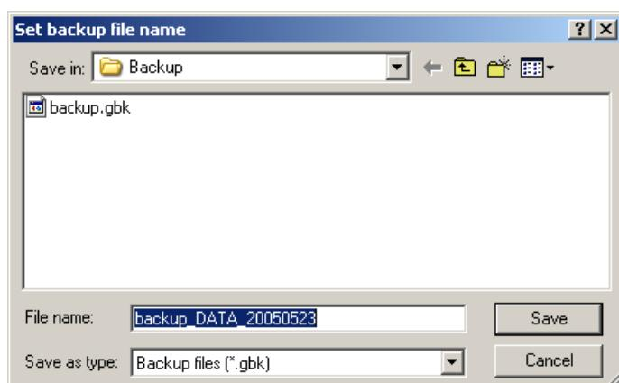
The current database is given a name and loaded to the panel **Backup** in GBK format using the function key **Save**.
