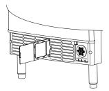
**UP Models: Air Filter Location** (insert mesh end first)
