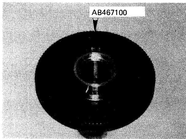
5-6. Remove knob (AB467100) by rotating it clockwise (direction of the arrow).
