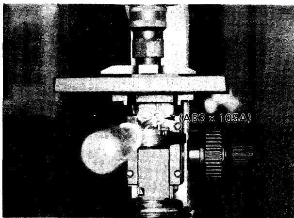
7-1-4. If the reading exceeds tolerance, adjust the tilt of condenser C2-CH carrier by loosening 4 clamping screws (AB3 x 10SA), tilting the entire assembly accordingly and tightening the 4 clamping screws.
