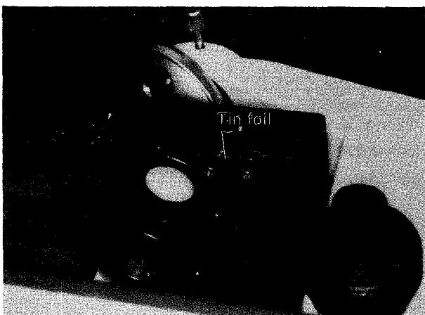
7-2-4. If the reading exceeds tolerance, adjust the tilt by inserting a piece of tin foil between the stage (AA871800) and the substage block (AB469400).
