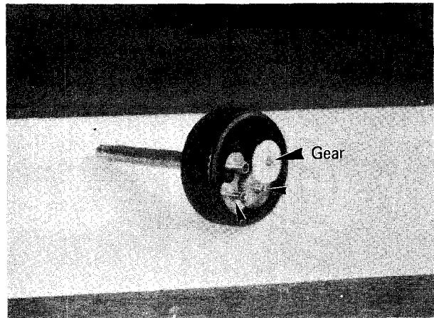
4-11. Remove the gears.
