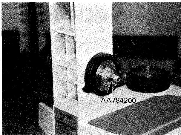
4-9. Pull out the right coarse focus knob in the direction of the arrow.
