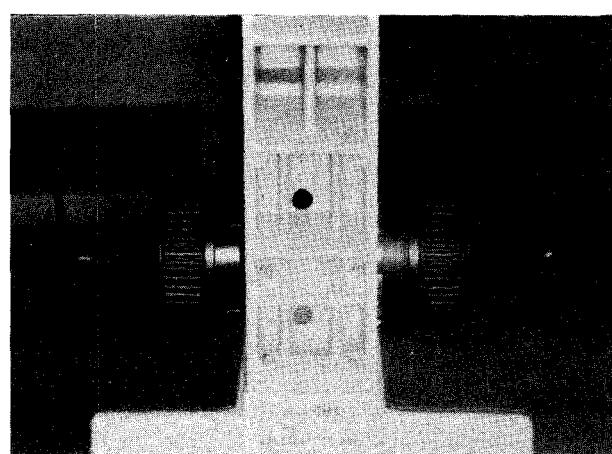
3-3-3. Tighten screw (AB3 x 8SA) which holds right and left hand focusing knobs.
