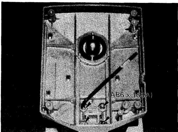
4-16. Assemble arm (C2-AS) and base (C2-BS) with 4 clamping screws (AB6 x 16SA).
