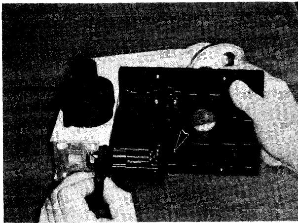
3-10. Remove the condenser carrier (C2-CH) from the arm (C2-AS).
