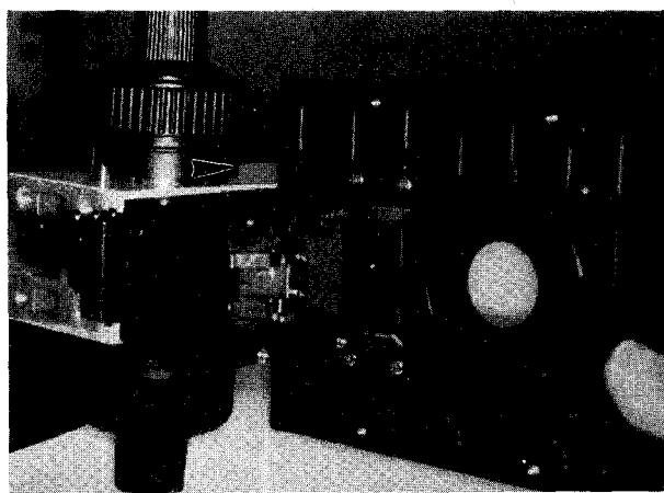
4-4. Lay down the microscope frame on its side and mount the condenser carrier following the direction of the arrow.
