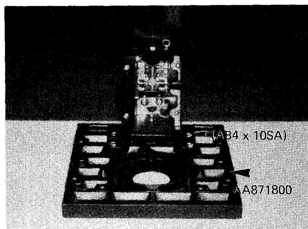
3-12. Release the stage (AA871800) by removing 4 screws (AB4 x 10SA).
