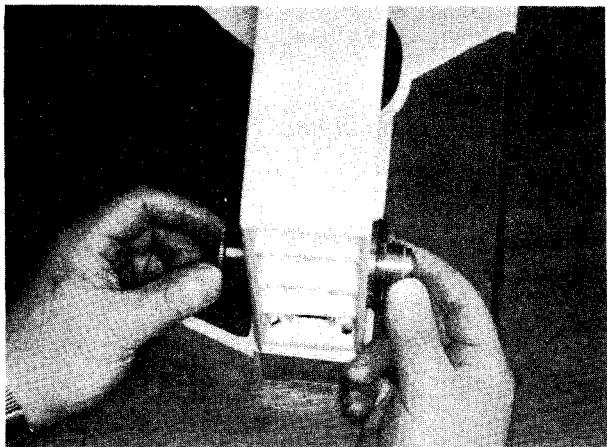
1-2-6. Put the arm in its original upright position and adjust the pinion shaft and the nut.
