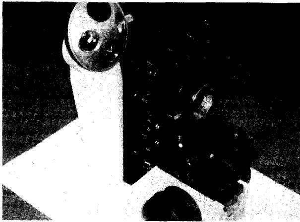
4-15. Check vertical movement of the condenser carrier.
