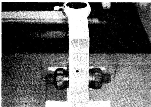
4-2. Remove the screws (AB3 x 8SA) which are holding the left and right knobs for the fine focus adjustment (AB059300/AB467500).
