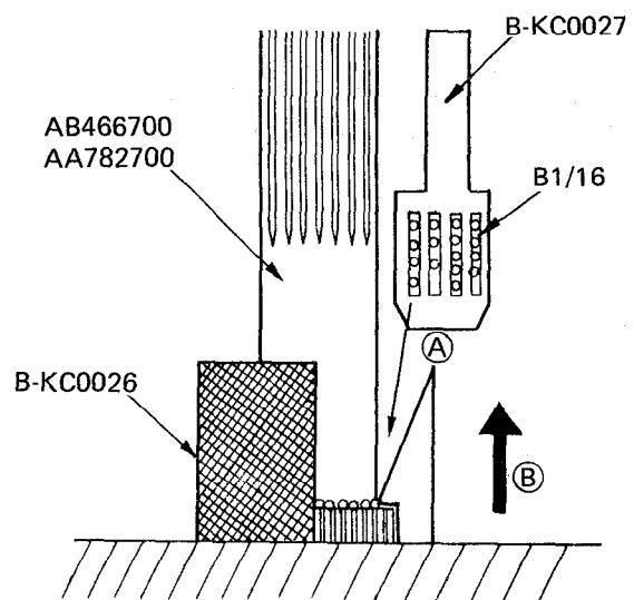
1-2-2. Fit 30 balls B1/16 around the pinion shaft.
