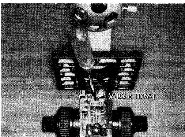
3-9. Remove 4 screws (AB3 x 10SA) from underneath the condenser carrier (AB468800) and release the guide (AB468600) and the block (AB009700).
