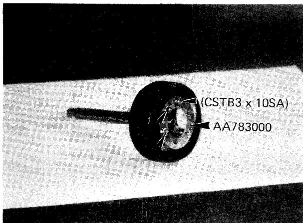
3-1-2. Mount plate (AA783000) with 3 screws (CSTB3 x 10SA).
