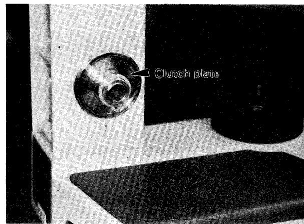
2-1. Mount the clutch plate on the pinion assembly.
