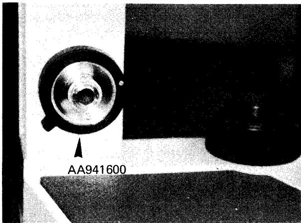
5-9. Remove the clutch plate.
