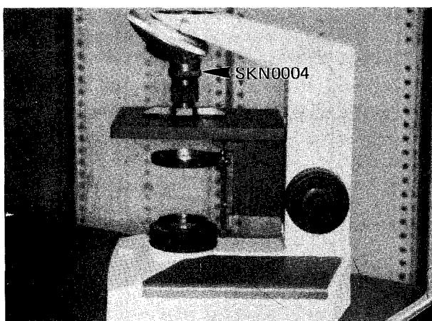
7-2-2. Rotate the jig (SKN0004) to bring it parallel to the Y-direction. Bring stage upwards until bottom surface of jig contacts stage surface.
