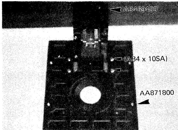
4-2. Mount the leaf spring (AB469500) on the stage bracket with 2 screws (CUK3 x 6SA).
