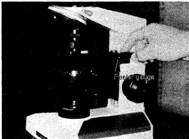
7-2-3. Check for equal clearance between the jig and the stage surface with feeler gauge (OT0317) at the front or back end. Maximum tolerance between stage and jig = 0.15 mm.
