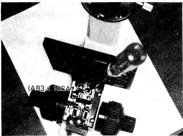
4-6. Check vertical movement of the coarse focus adjustment guide.
