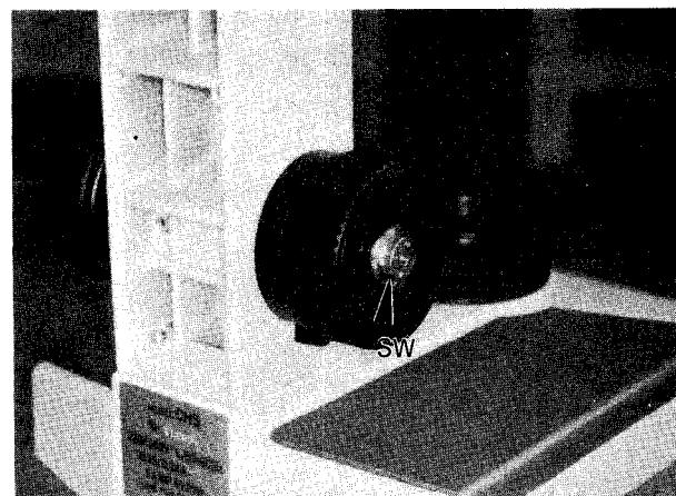
3-2-7. Place the spring washer on the shaft.
