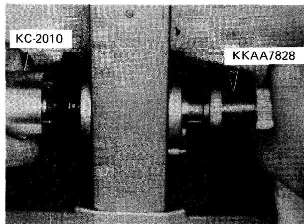
5-1. Place tools KC-2010 and KKAA7828 on the right gear (AA782700) and the left nut (AA782800) respectively, then rotate them counter-clockwise and remove the nut.
