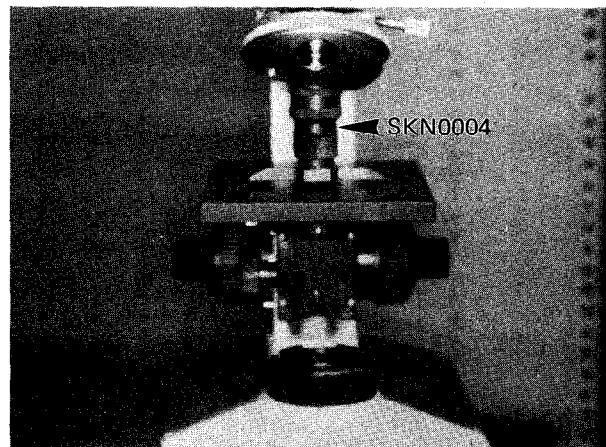
7-1-2. Rotate the jig (SKN0004) to bring it parallel to X-direction. Bring stage upwards until bottom surface of jig contacts stage surface.
