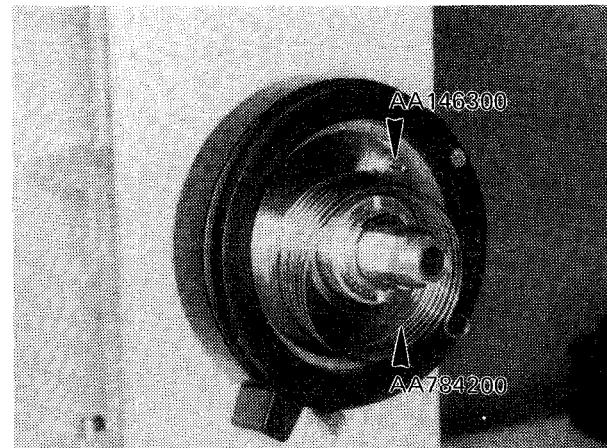
3-2. Assemble the left hand knob assembly of the coarse focus unit.
