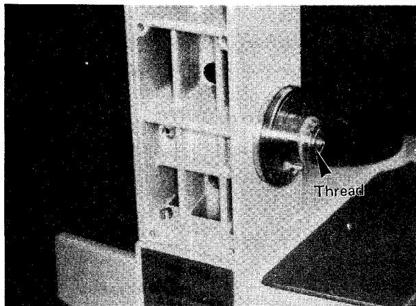
1-2-7. Apply glue (OT1027) on the threads of the nut.
