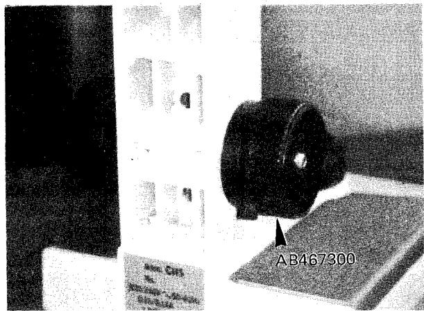
3-2-5. While holding left coarse handle AB467300 still with your hand, push the right coarse handle in the arrow direction.
