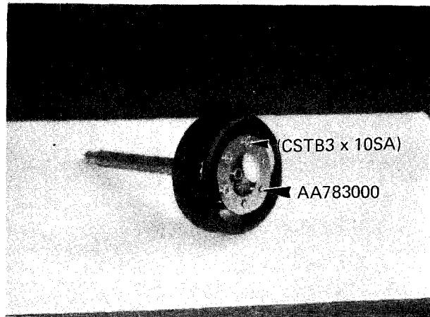
4-10. Remove plate (AA783000) by removing 3 screws (CSTB3 x10SA).
