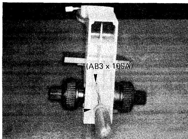
3-8. Remove the rack for coarse focus adjustment (AB469300) by removing 2 screw (AB3 x 10SA) from the back of the arm.
