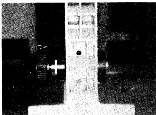
3-1-4. Affix the right hand knob assembly on the microscope arm.
