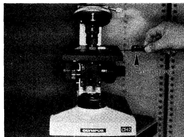
7-1-3. Check for equal clearance between the jig and stage surface with the thickness gauge (OT0317) at the left or right end. Maximum tolerance between stage surface and jig surface = 0.15 mm.
