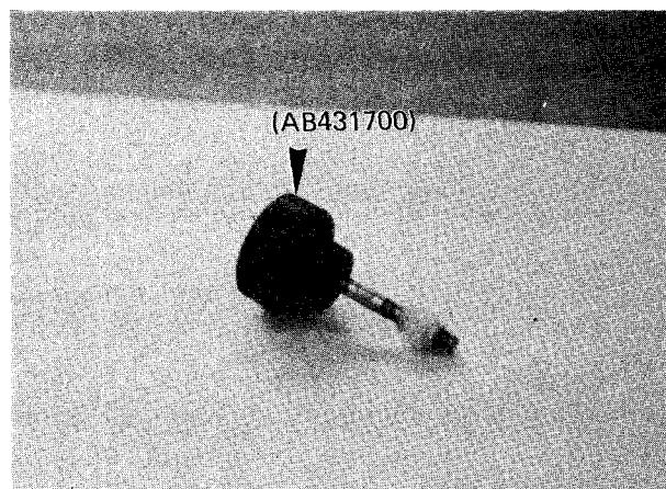
3-6. Remove substage knob assembly (AB431700).
