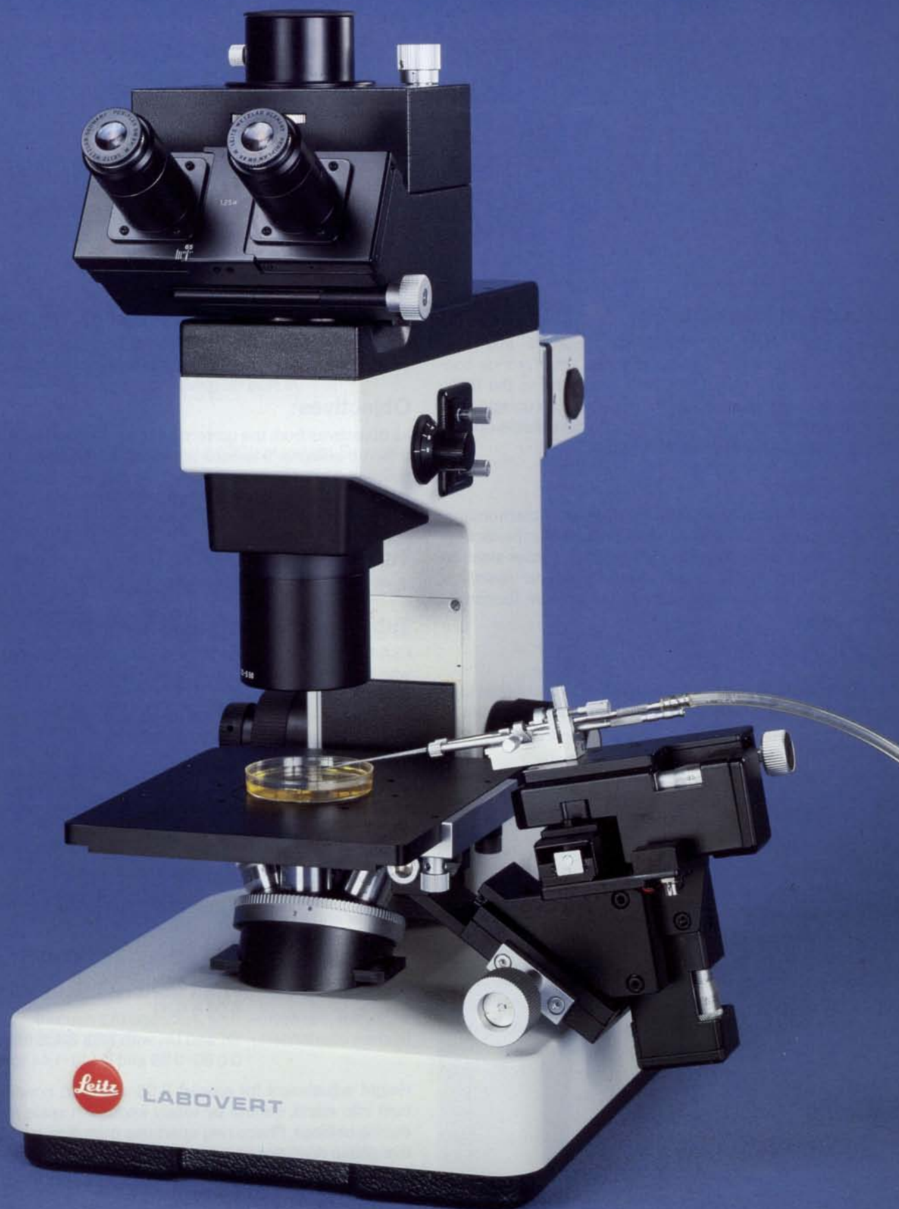
LABOVERT with FSA-GW-R tube, S 50 condenser and micromanipulator
