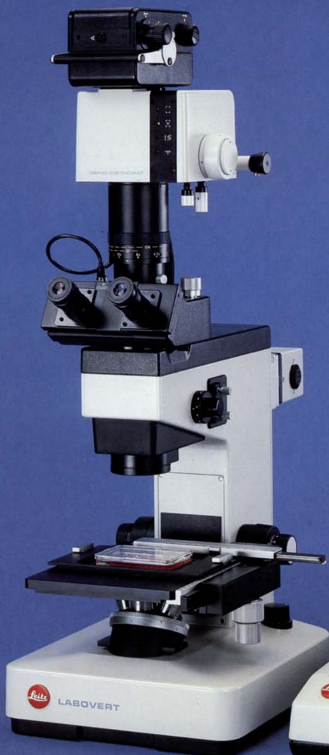
VARIO ORTHOMAT 2 and inset WILD MPS camera systems with 24mm x 36mm film magazine.
