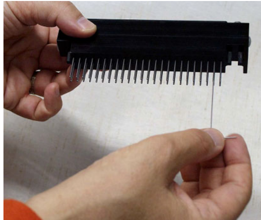
Fig. 7.2 Cleaning the aspiration needles
