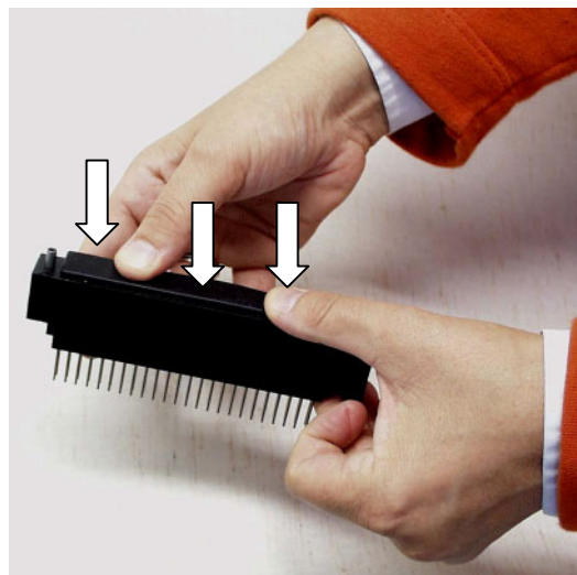
Fig. 7.4 Remounting the silicon top seal (B)
