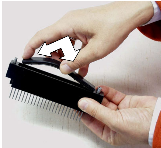
Fig. 7.3 Remounting the silicon top seal (A)
