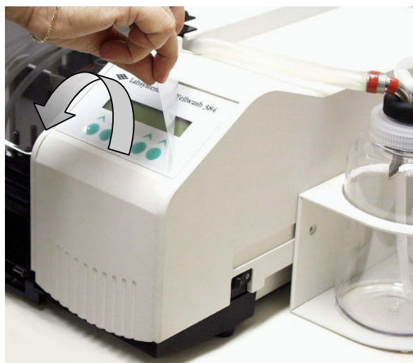
Fig. 5.6 Removing the adhesive tape on the keypad and display
