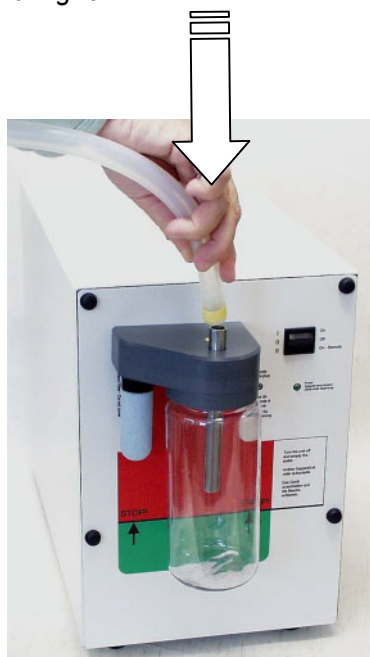
Fig. 5.10 Connecting the tubing (yellow) to the vacuum source
