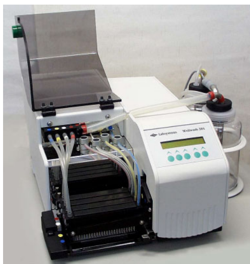
Fig. 4.2 Wellwash 384 front view with the aerosol cover open
