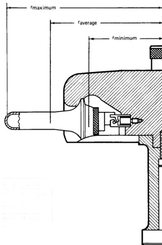
**Figure 3-1.** AH-629 Rotor Cross Section Showing Radial Distances
