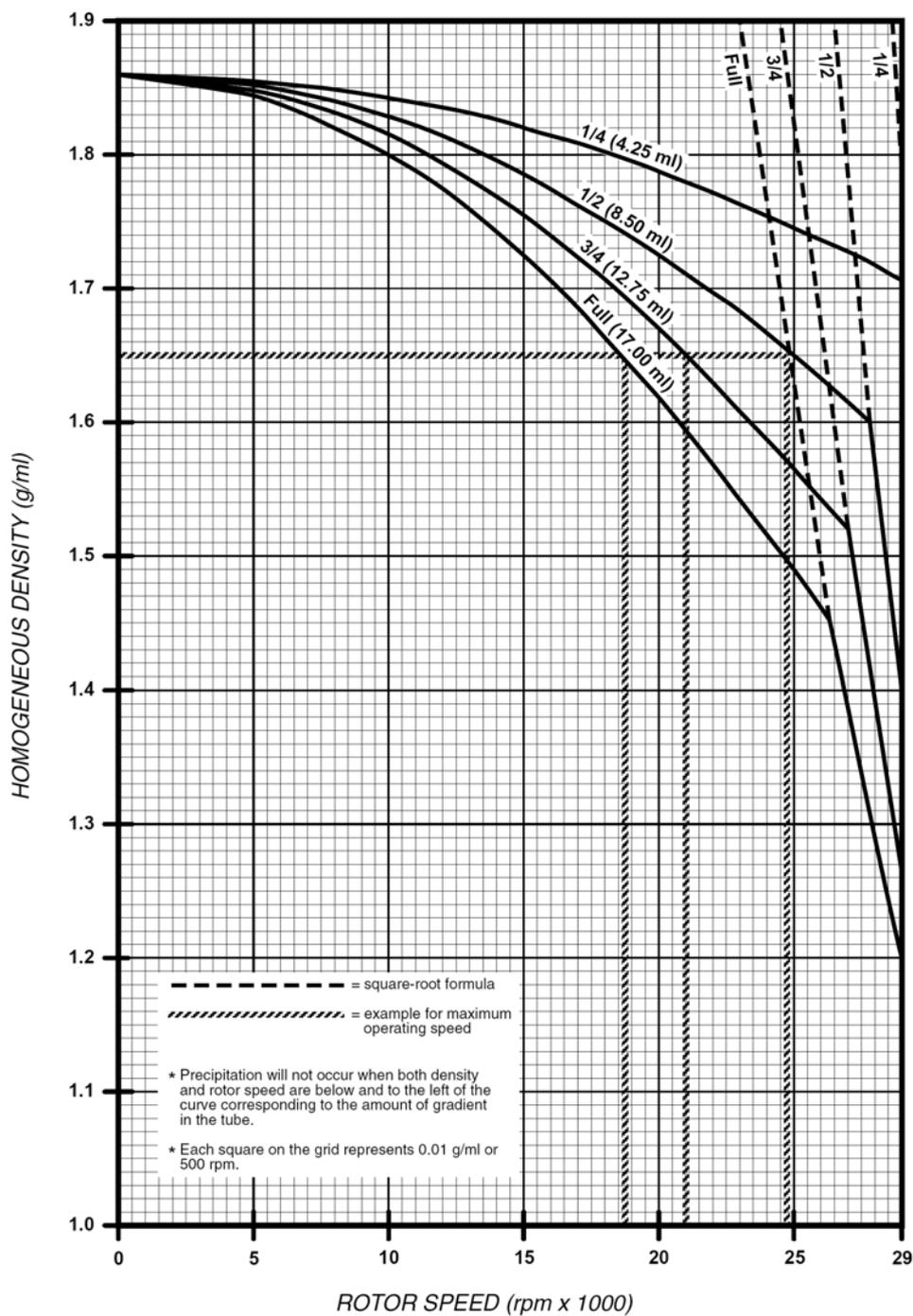
Figure 2-7. CsCl Precipitation Curve, 17 ml Buckets, 25°C
