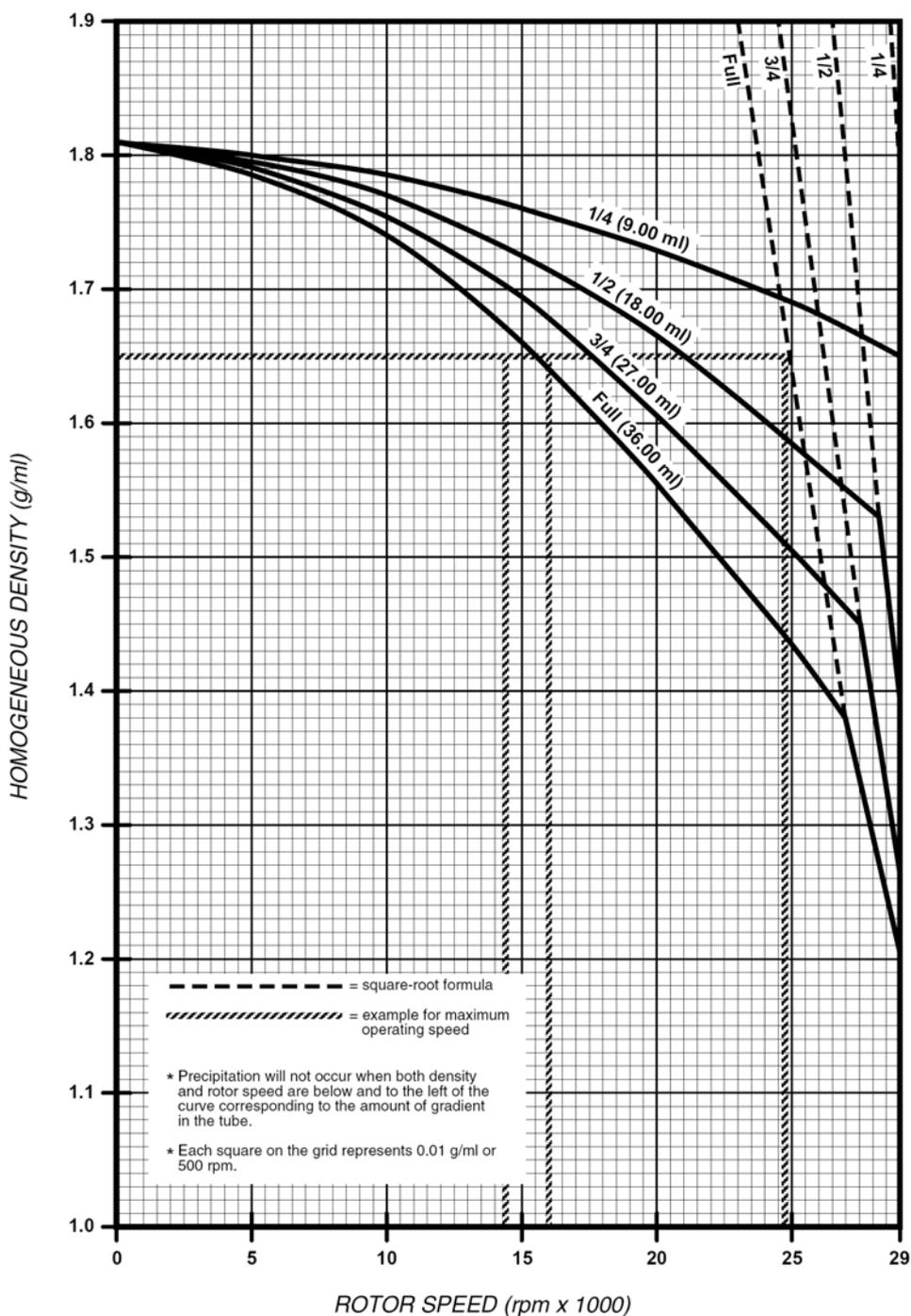
Figure 2-5. CsCl Precipitation Curve, 36 ml Buckets, 5°C
