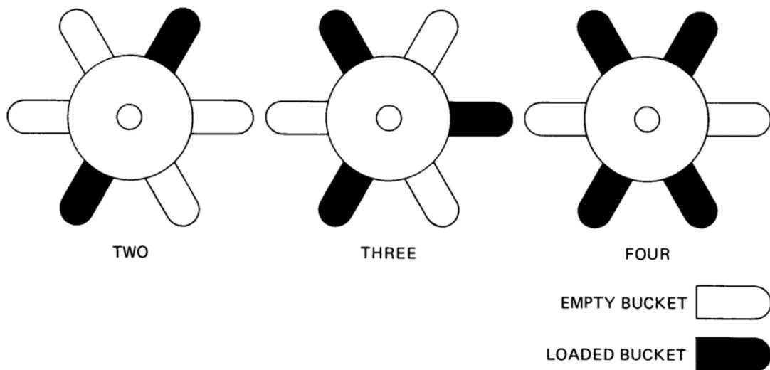
**Figure 3-3.** Rotor Balancing
