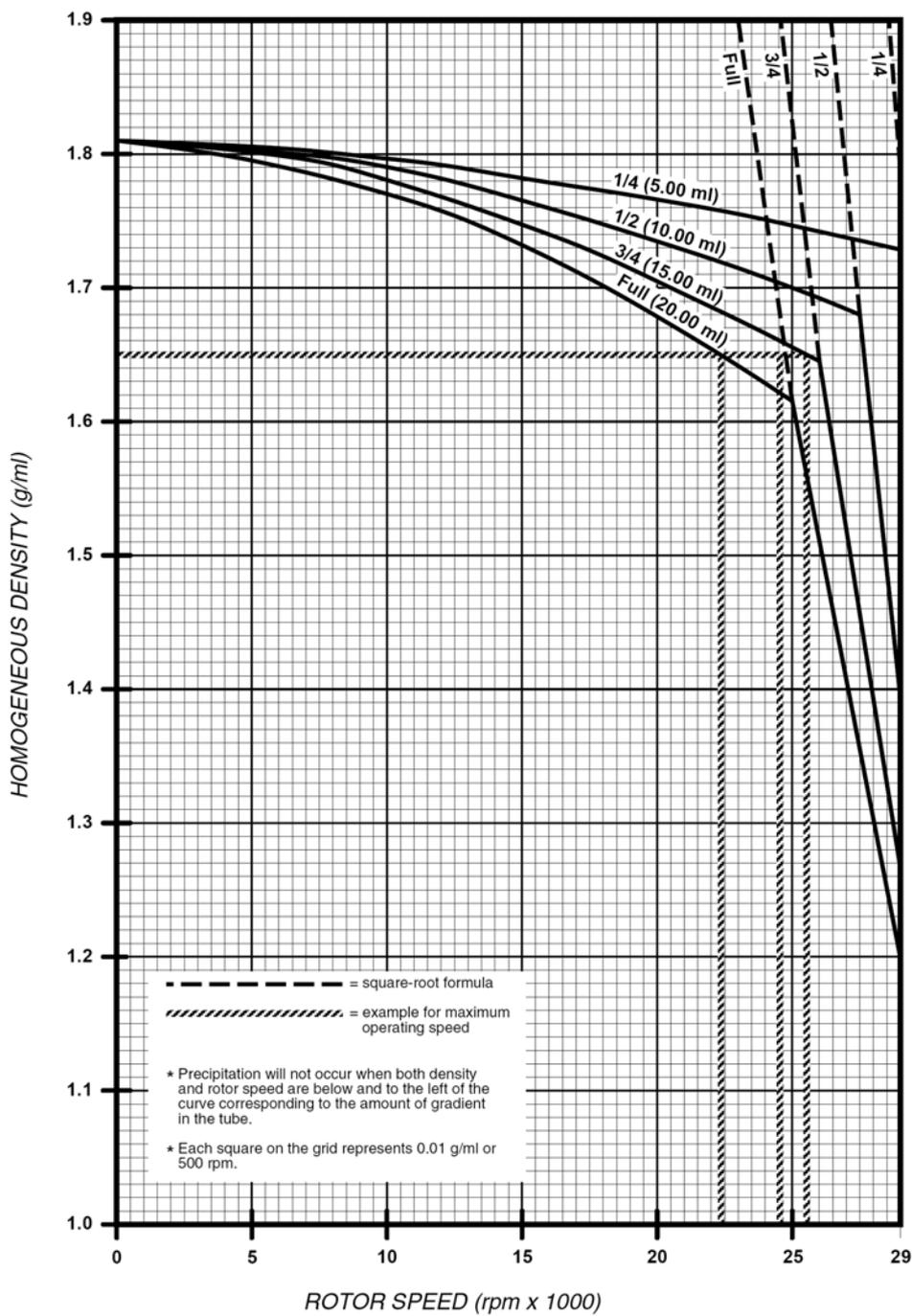
Figure 2-3. CsCl Precipitation Curve, 20 ml Buckets, 5°C
