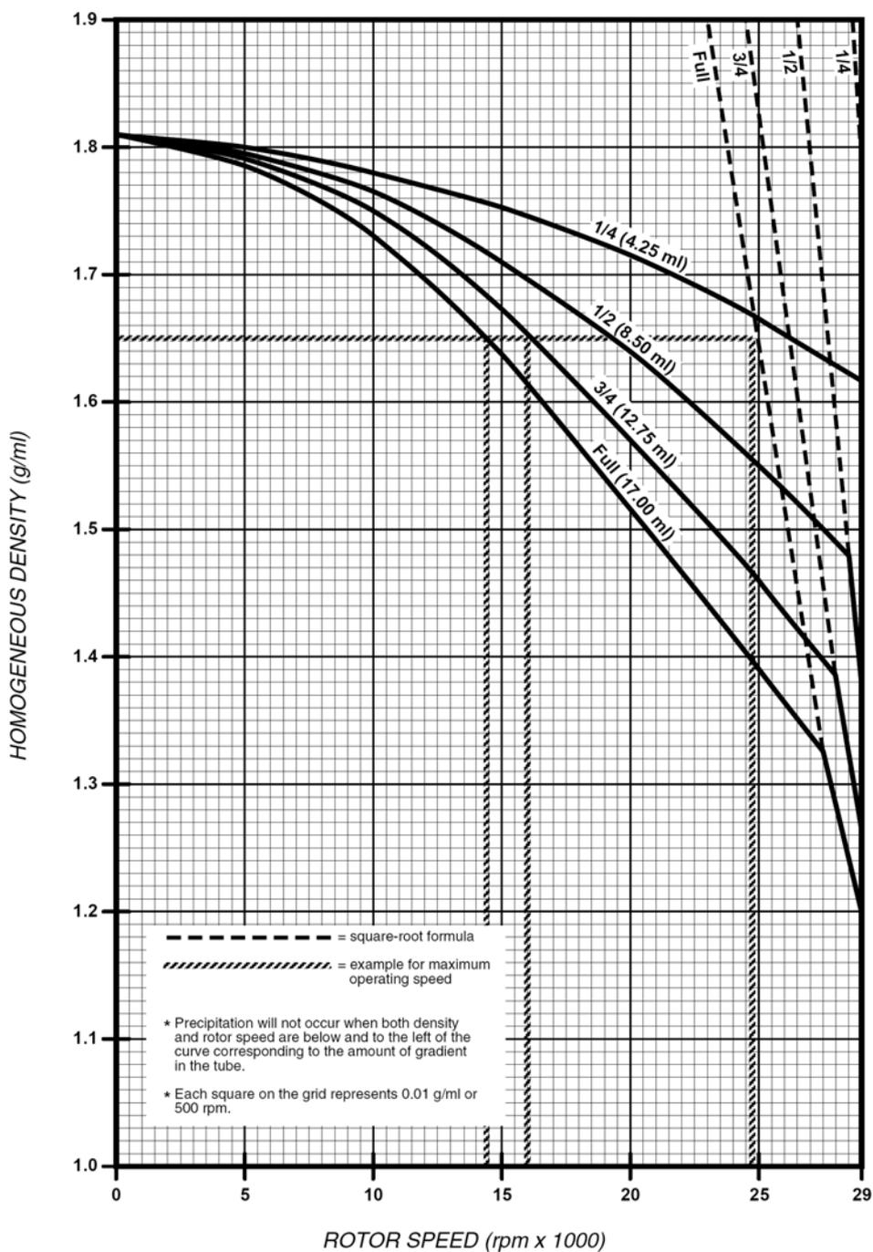
Figure 2-1. CsCl Precipitation Curve, 17 ml Buckets, 5°C
