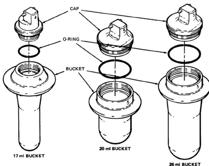
**Figure 3-2.** Cap and Bucket Assembly
