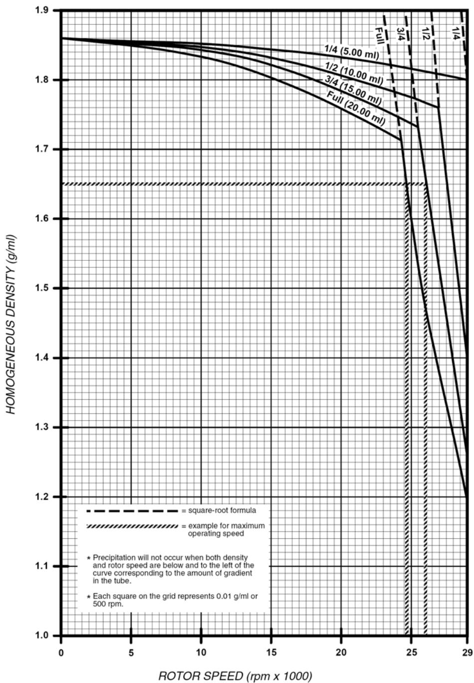
Figure 2-9. CsCl Precipitation Curve, 20 ml Buckets, 25°C
