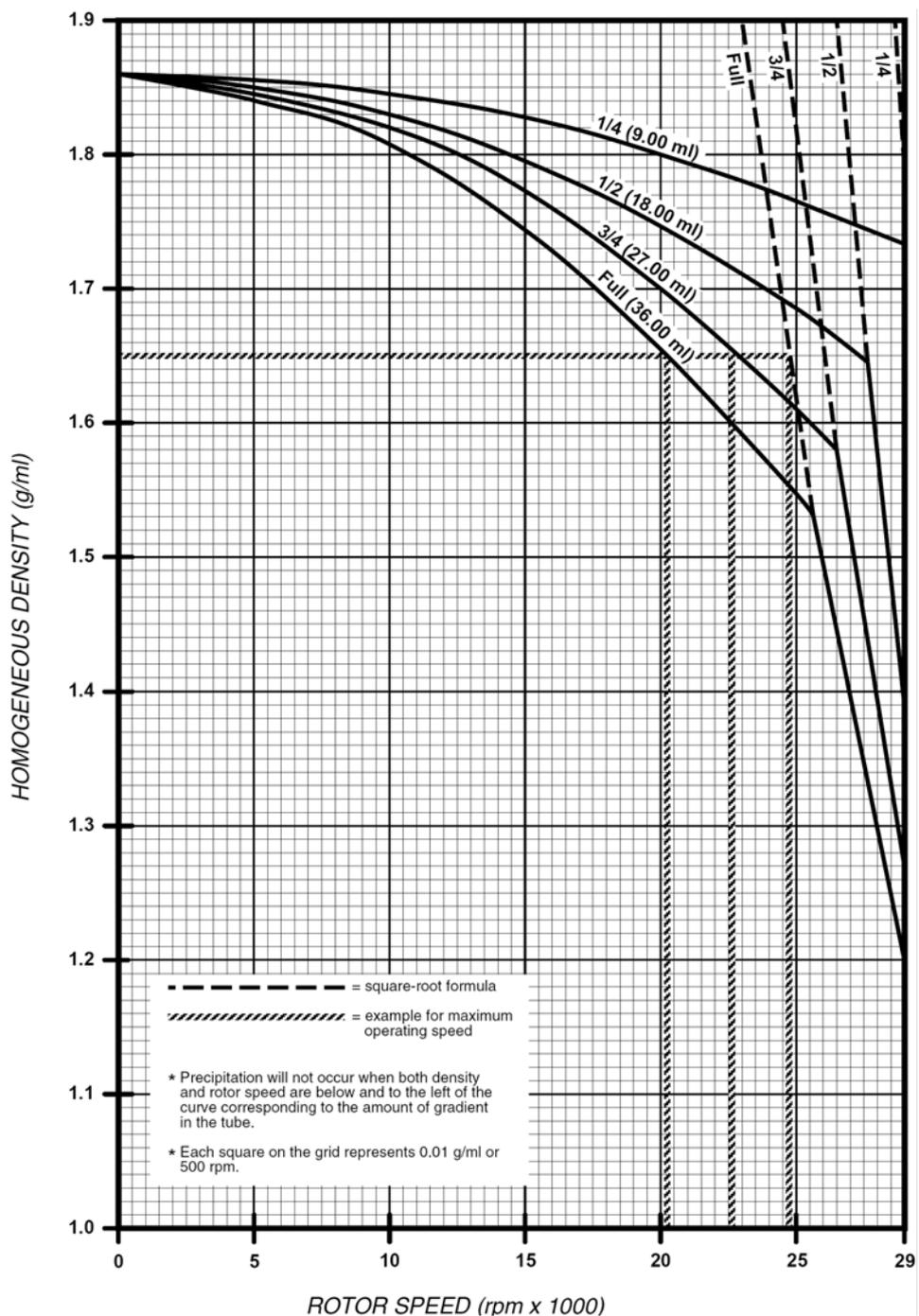
**Figure 2-11.** CsCl Precipitation Curve, 36 ml Buckets, 25°C
