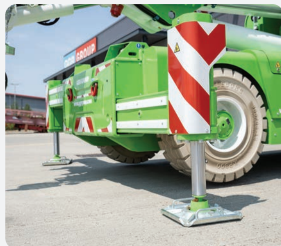
With four deployable outriggers, stability is optimised for when lifting a load and when slewing the turret.
