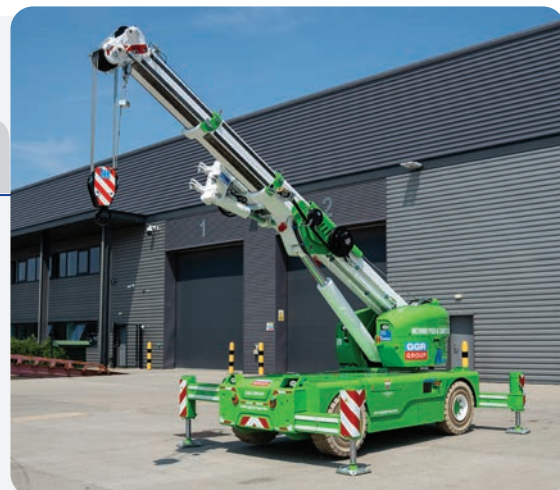
The MC100RE main boom can reach a max lifting height of 10.2m when using the main hook. Alternatively, operators can use the full winch system to allow lifting from different levels/floors.
