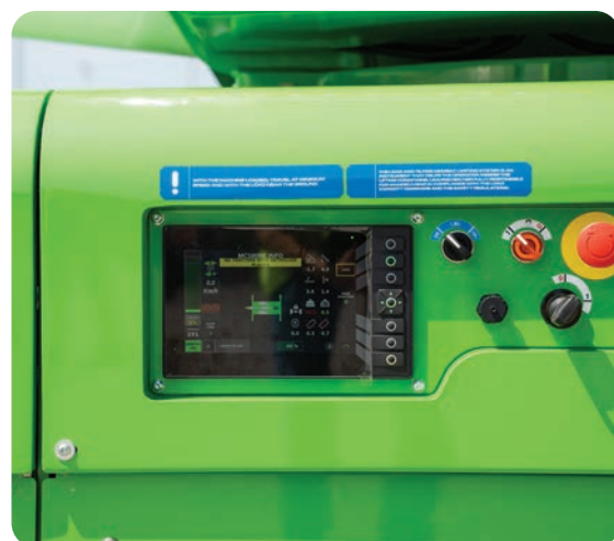
While information is supplied to the operator via the radio remote control, on the machine there is a handy digital display showing all relevant information.
