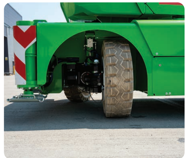
180° rear steering allows the MC100RE to manoeuvre in the tightest areas typically found on construction sites or in factories, warehouses and production lines.
