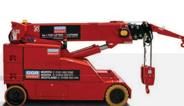
Optional 4.2t max capacity winch
