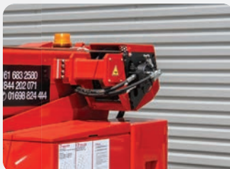
Optional 4.2t max capacity winch
