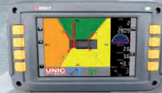
Variable Footprint safe load indicator
