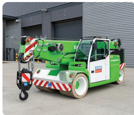
The MC180 can be fitted with either a full-winch system allowing a hook block attachment, or a hook only. Both options can also be used on the hydraulic jib.
