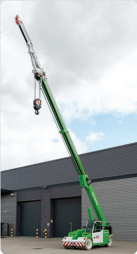
The hydraulic jib can be easily fitted and extended to increase the maximum lifting height.
