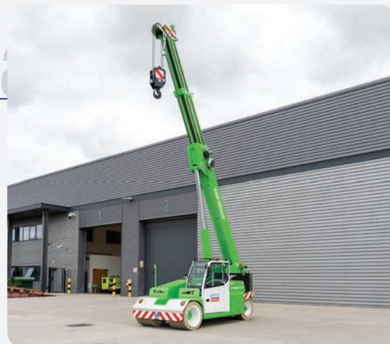
The MC180 Main Boom can reach a max lifting height of 11.6m when using the fixed hook. Alternatively, operators can use the full winch system to allow lifting from different levels/floors.
