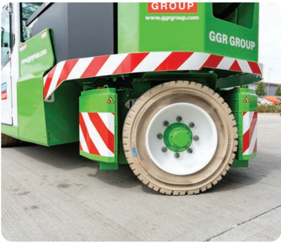
180° rear steering allows the MC180 to manoeuvre in the tightest areas typically found on construction sites or in factories, warehouses and production lines.
