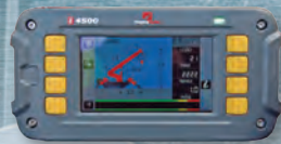
Safe load indicator
