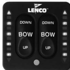
BOTH SIDES FAULT
