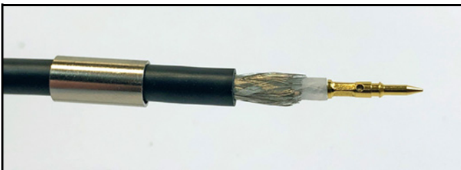
Figure 51: Center Pin Crimped in Place
