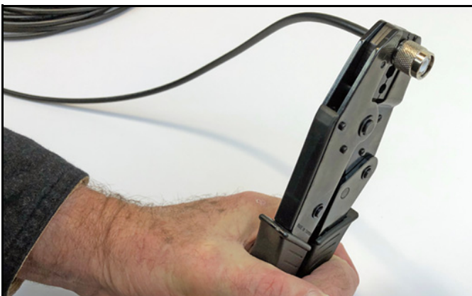
Figure 57: Crimping the Ferrule onto the Cable
