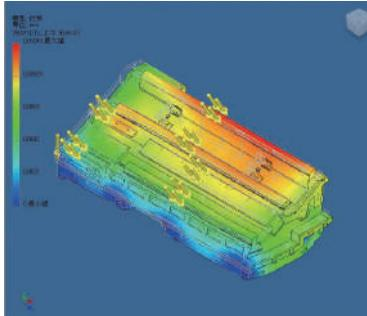
► By using Finite Element Methods ( FEM ), optimally reinforced ribbings are directly casted into the one-piece bed structure. Mechanical rigidity has been increased by more than 30% when compared to conventional designs.
