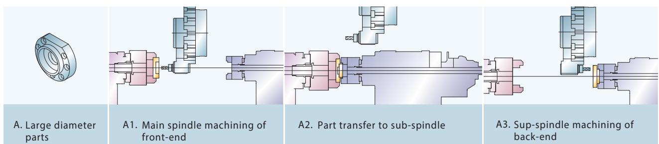
► With Ø 45 mm ( 1.77" ) bar capacity, the sub-spindle configuration is also ideal for machining long work pieces such as small diameter shafts. Both ends of the work piece can be supported by the main and sub spindles, allowing the middle section(s) to be accurately machined.
