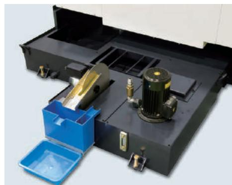
Separate coolant tank & Oil skimmer shown
