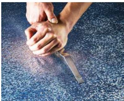
► Contact surfaces of all slides, headstock, turret, tailstock, and ball screw bearing housings with the machine bed are hand scraped to provide maximum assembly precision, structural rigidity, and load distribution.
