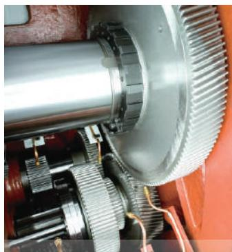
► The 2-speed, super heavy-duty gear head incorporates advanced mechanical designs. Mated with a 37 kW ( 30 min. ), a tremendous amount of low-end torque is provided to handle heavy material removal on large diameter parts.
