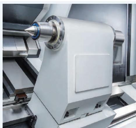
**Programmable tailstock design, both tailstock positioning and quill are programmable.**
