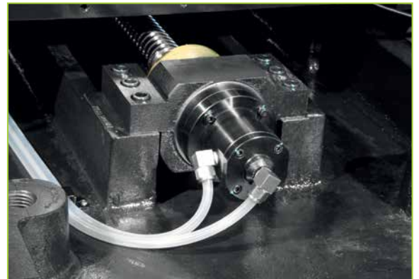
Oil cooling through ballscrew(Only available on VF1100)
