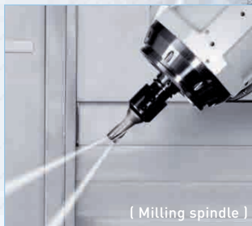
Coolant Through Spindle
