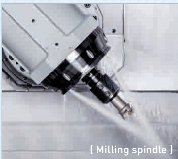
Coolant Nozzle Around Spindle
