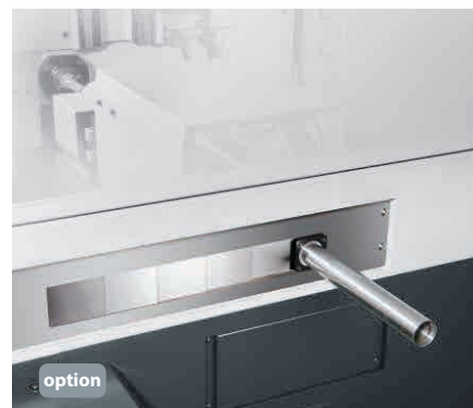
Long parts ejector
