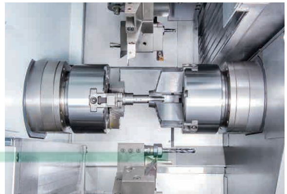
Twin spindles simultaneous part catching
