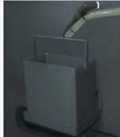
Built-in lub. oil collection system
