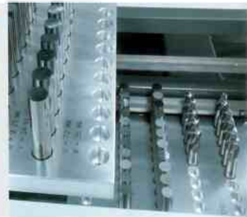
The pallets can also be fitted with tools of different lengths.
