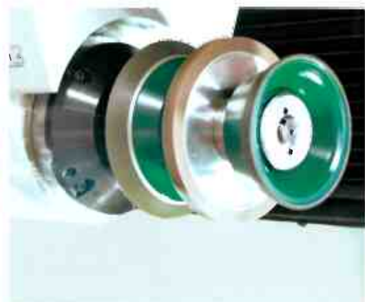
The second spindle end can be used to execute all grinding operations in the customary way.
