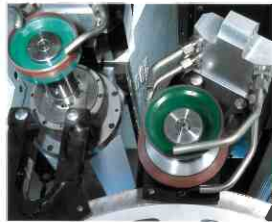
The grinding wheel set, including coolant feed, can be changed in less than 10 seconds.
