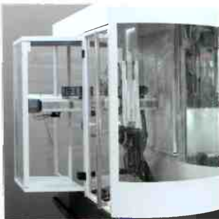
Helitronic Power with with machine-integrated Palett loader.
