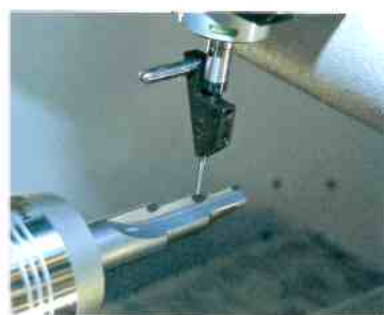
The automatic tool measurement and positioning device helps minimise downtime.
