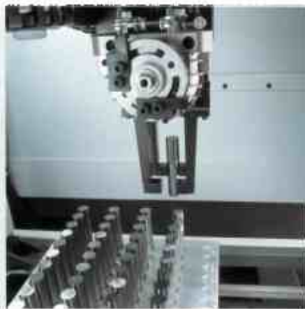
Lift loader: The machine can be loaded with up to three pallets stacked with blanks or tools of different lengths and dimensions for automatic machining.
