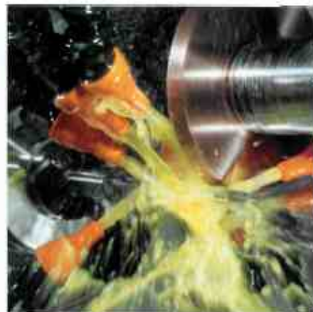
The temperature rises to over 8,000 °C at the surface of the disk electrode during rotational erosion.
