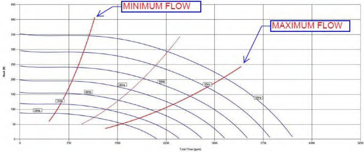
Figure 20: Sample Pump Curve
