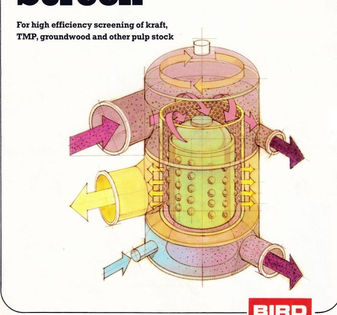
The Centrisorter Pressure Screen is the first pressurized screen developed for use on groundwood, kraft and other pulp. It also has wide application in screening high consistency stock in the paper mill. The Centrisorter Screen operates at higher consistency and with higher efficiency than conventional screens. It has been tested and sold for primary and rejects use on news and roto grade grinder groundwood, refiner groundwood, bleached and unbleached kraft, and on waste stocks.
