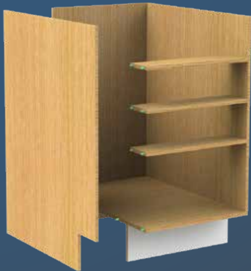
Drilling & Dowel Inserting
